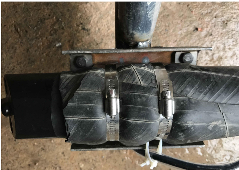
Fig. 34 Fixing the Sensor on Bracket
