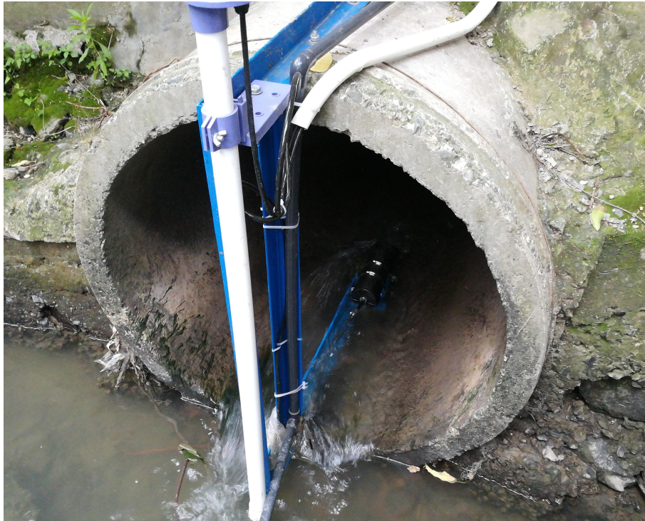
Fig.: 28 Installation Diagram of \Phi 800 mm Pipe
